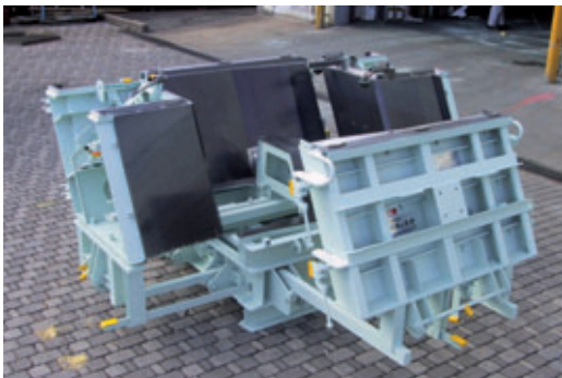
Fig. 3a, 3b: Examples of retaining wall molds used in Japan
