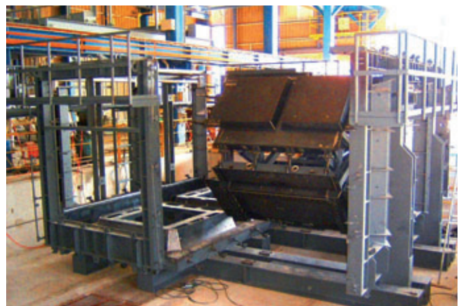
Fig. 4: Precast concrete form/mold for the production of the precast lavatory
