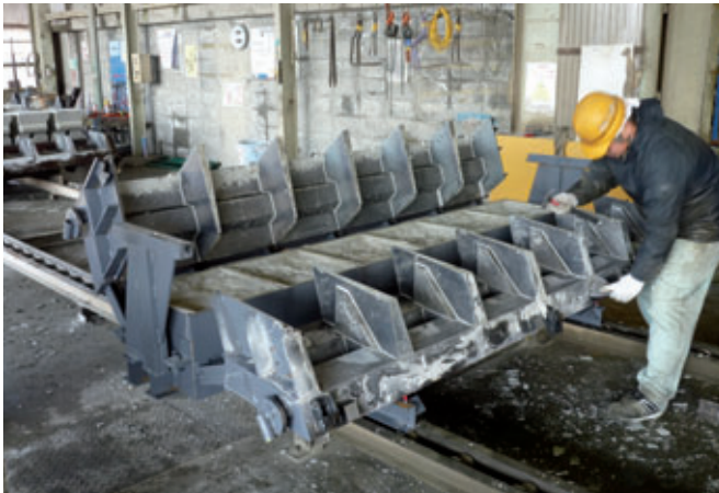
The moulds made by Toyota Forms can be operated easily by one person.
