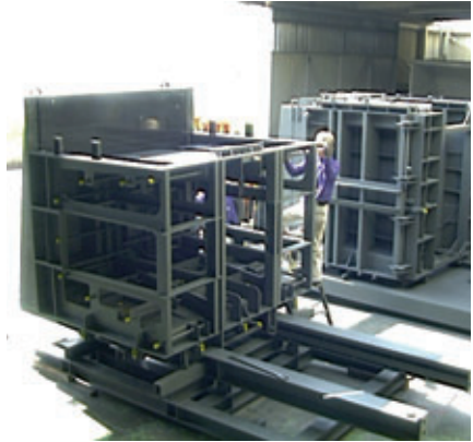
Fig.7: Adjustable mold for the Road L retaining wall.
